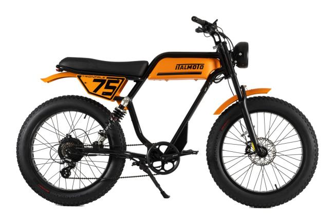
**Full recharging** takes about **4 to 6 hours**. The **battery** provides a **maximum range** of **80 km**, which varies depending on factors such as range (the weight of the driver or driver + passenger), type of route (climbs require more effort) and weather conditions.
